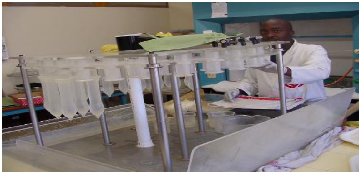
Figure 15: Every condom is tested electronically for pinholes at the factory level. Quality is emphasised at every stage of the manufacturing process
