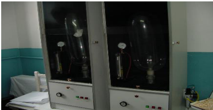
FIGURE 14: CONDOMS INFLATED WITH AIR TO TEST THE STRENGTH OF THE LATEX – CONDOMS NORMALLY BREAK AT 34 LITRES OF AIR
