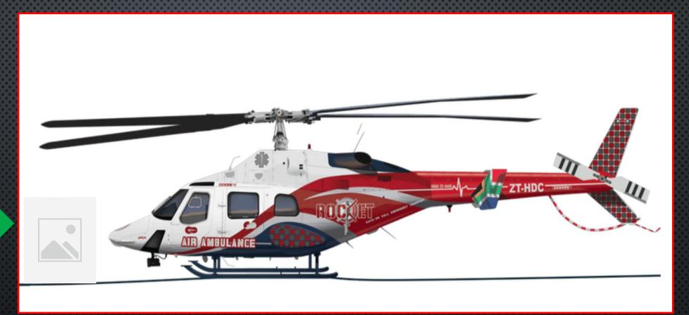
Approach the helicopter from the front, in a crouched position when the blades are turning, in view of the pilot!
